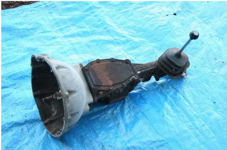
4-speed manual gearbox (goes with 6-cylinder motor)
